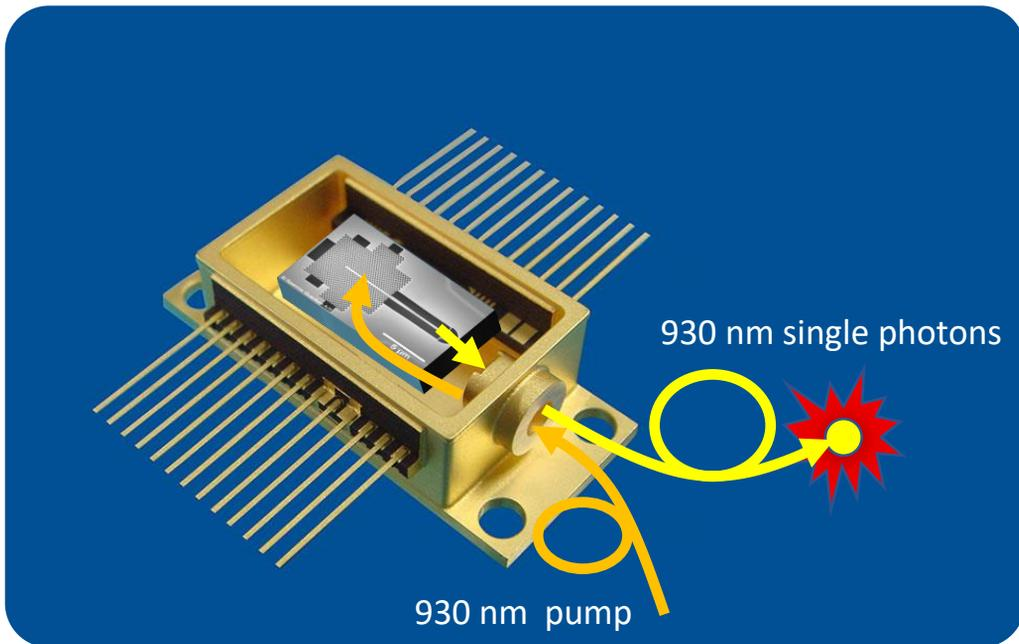
Fig. 5. Schematics of the fiber coupled housing of the SPS chip. The chip is placed on a metal plate which allows for coupling to a cryostat. Two fibers are tapered to the chip, for providing the excitation signal and the other fiber collecting the output photons.
