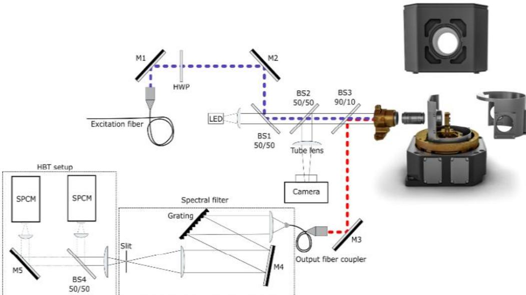
Figure 4: Typical optical setup around the SPS free space component. The component is placed in the cryostat at the right. A laser excitation source is coupled perpendicular to the component. The emission signal is collected from the same path, and an optical setup ensures the separation between the excitation and emission signal, as well as filtering the single photon source from excitations from other quantum dots on the chip.
