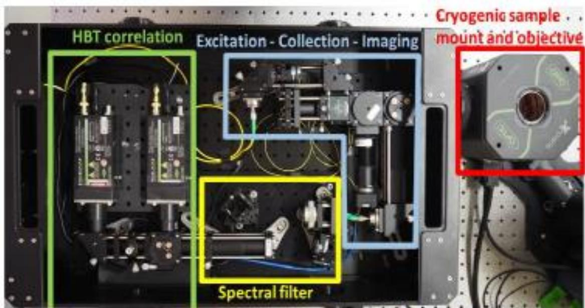
Fig. 7 Top view of the Sparrow SPS 930 nm module.
