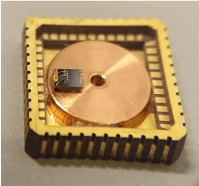
Fig. 3. Free space housing of the SPS chip. The chip is placed on metal plate which allows for coupling to a cryostat. In the free space version a transparent top lid allows for in and outcoupling of an optical signal. The chip is placed at an angle relative to the housing window which allows for in and outcoupling through the same optical path perpendicular to the housing. The table shows the specifications for the component.
